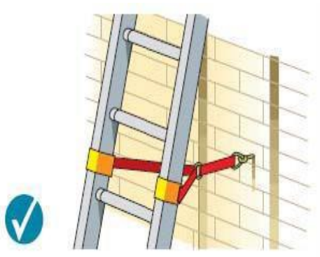
Tying near the base
